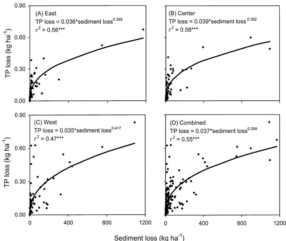
Fig. 6. Relationships between sediment loss and total phosphorus loss for (A) east, (B) center, (C) west watersheds, and (D) all three combined. \*\*\* Significant at the 0.001 probability level.
