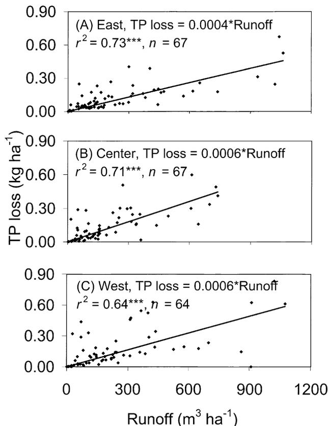
Fig. 4. Relationships between runoff volume and total phosphorus loss for (A) east, (B) center, and (C) west watersheds. \*\*\* Significant at the 0.001 probability level.
