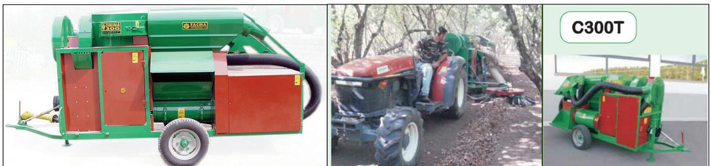
*The C300T mechanical vacuum harvester hard at work. When used by chestnut growers, it can sweep and vacuum in over 1,300 pounds of chestnuts per hour. This harvester also removes the spiny bur from each chestnut, and can help minimize labor costs for chestnut growers. Photos courtesy of FACMA.*
